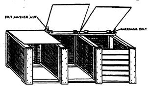
A wood and wire three-bin turning unit can be used to compost large amounts of yard, garden, and kitchen wastes in a short time. Although relatively expensive to build, it is sturdy, attractive, and should last a long time. Construction requires basic carpentry skills and tools.
