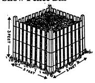
A snow fence bin is simple to make. It works best with four posts pounded into the ground for support.
