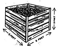
A wooden box bin can be built inexpensively using wooden pallets. Or you can use lumber to make a nicer looking bin. The costs will vary, depending on whether you use pallets or new lumber. Used pallets are often available from manufacturers and landfills.
